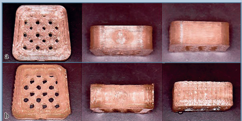
Fig. 4 Experimental cage samples: a – with layer orientation parallel to the printing table (as built); b – with layer orientation perpendicular to the printing table (transverse)
