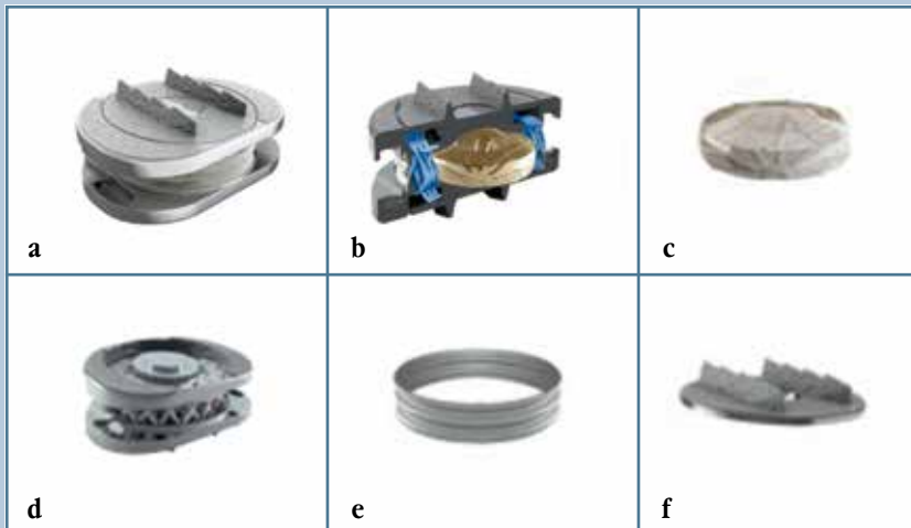
Fig. 5 The M6-L artificial disc [10]: a – a general view; b – view of prosthesis in section; c – artificial nucleus pulposus; d – kinematic part of the disc assembly (nucleus pulposus, artificial fibrous ring, internal endplates); e – polyethylene sheath; f – external titanium endplate
